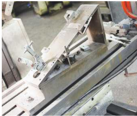
▲ Shop-made jigs play their part for some of the milling operations. This one...
